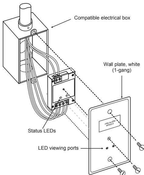
**SIGA-MCT2:** mount the UIO motherboard inside a suitable EDWARDS enclosure with screws and washers provided. Plug the SIGA-MCT2 into any available position on the motherboard and secure the module to the motherboard with the captive screws. Wiring connections are made to the terminals on the motherboard (see wiring diagram). UIO motherboard terminals are suited for #12 to #18 AWG (2.5 mm<sup>2</sup> to 0.75 mm<sup>2</sup>) wire size.
